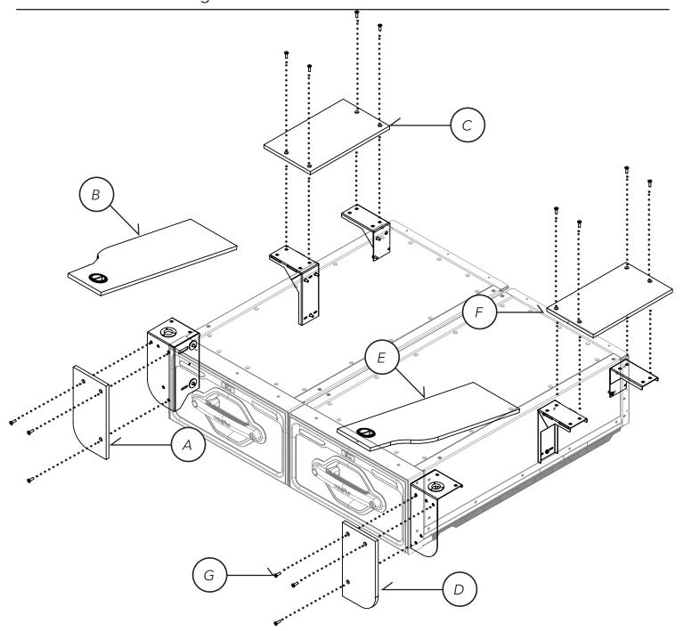
STEP 5 - Wing Kit Panel Assembly:Securely Assemble the Wing Kit Panels to the Brackets
