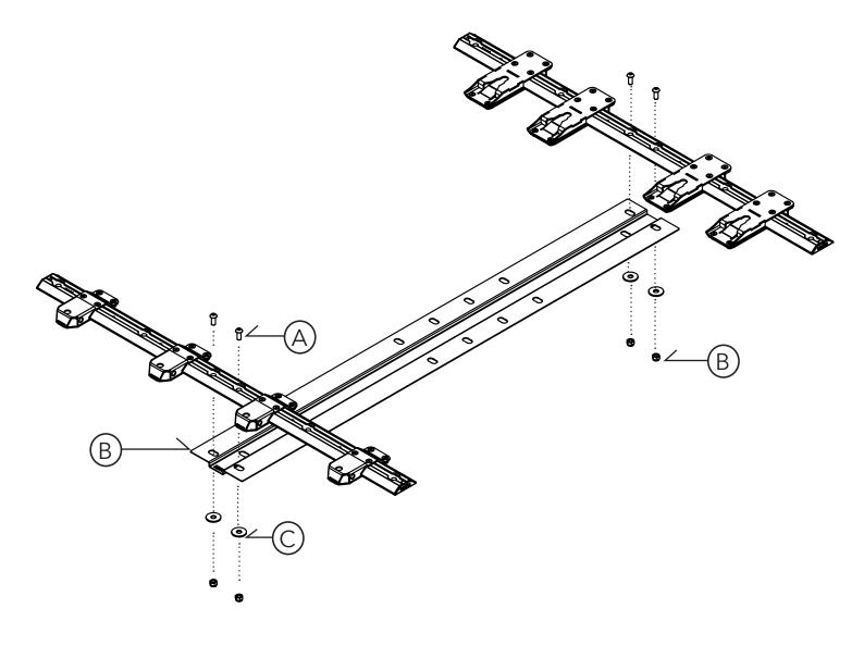
STEP 14 - Assemble the Centre Rail of the 1400 Mounting Platform to the pre-assembled cross rails.
