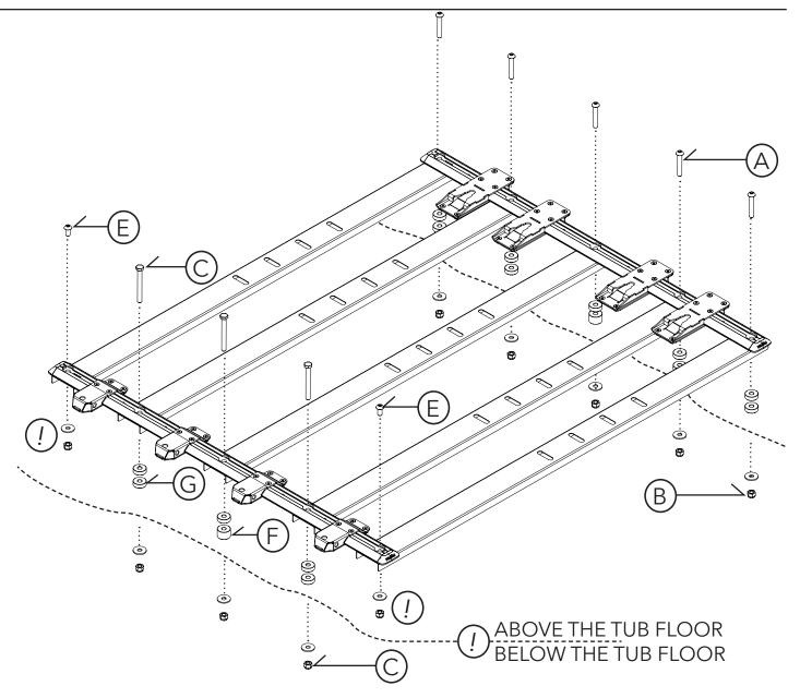
STEP 14 - Secure the 1400 Mounting Platform to the Ute Bed:
