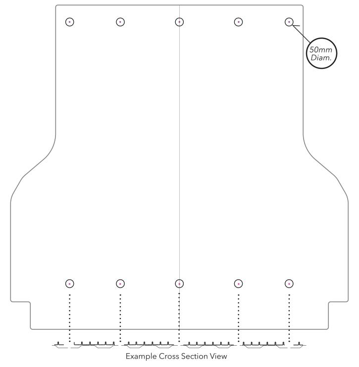
NOTE: Tub-liners can vary significantly. The KUFU Mounting Platform should be securely attached to the steel floor of the ute tub. Removing the tub liner material allows space needed to raise and level the Mounting Platform above different liner profiles.
