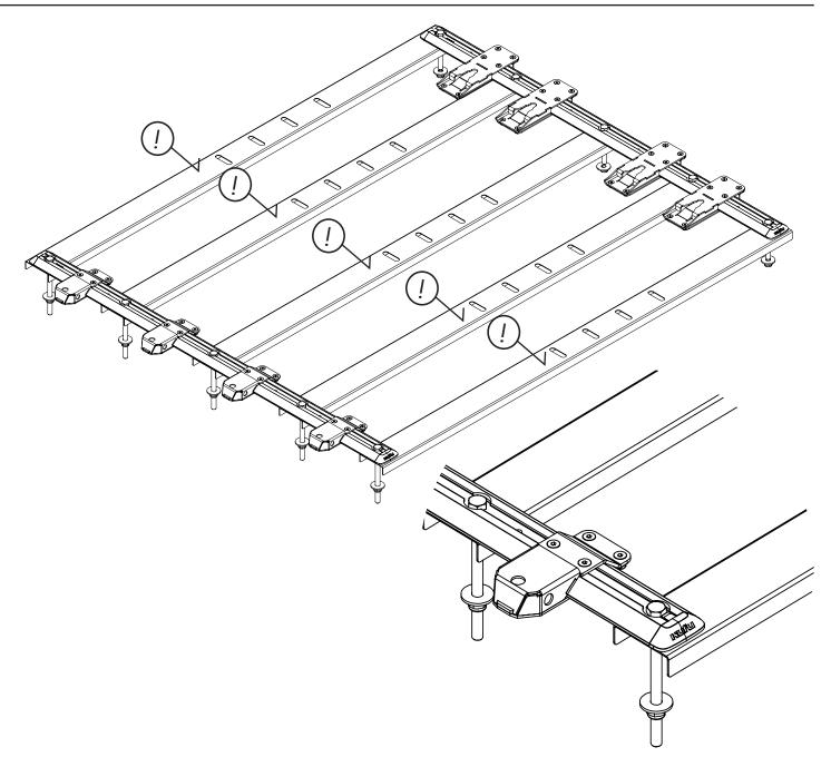
STEP 15 - Fasten the 1400 Mounting Platform to the Ute Bed:
