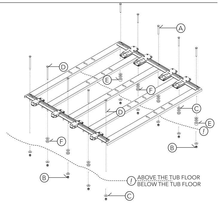
STEP 14 - Secure the 1400 Mounting Platform to the Ute Bed:
