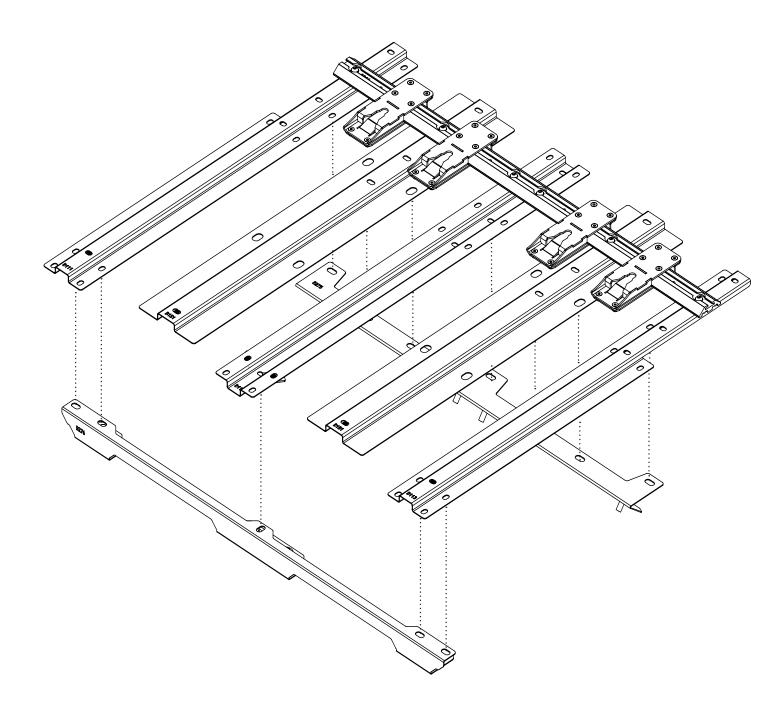
STEP 10 - Alignment of Mounting Platform to the Vehicle Floor Brackets
