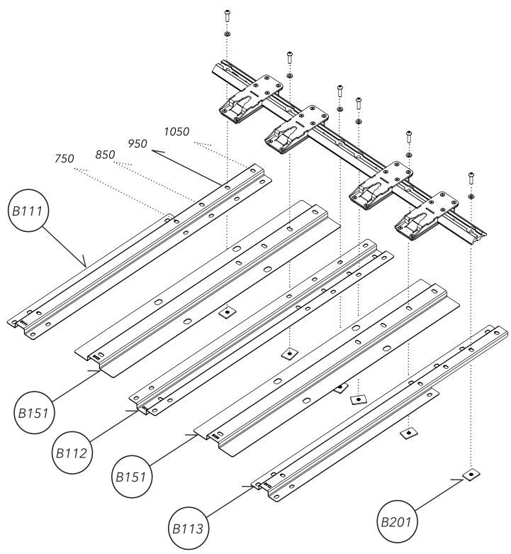
STEP 9 - Partial Assembly of the Mounting Platform Frame:
