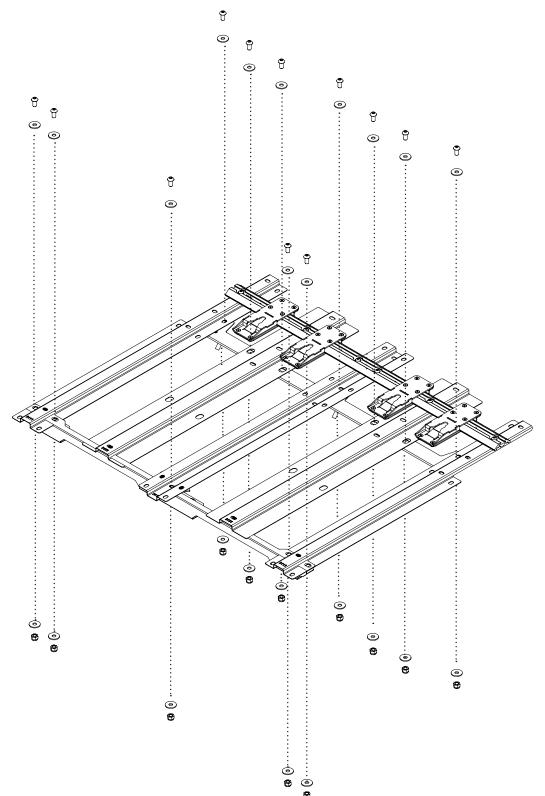
STEP 11 - Assembly of Mounting Platform to Vehicle Floor Brackets
