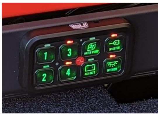
Kufu SPARK, Smart 8 Switch Panel
